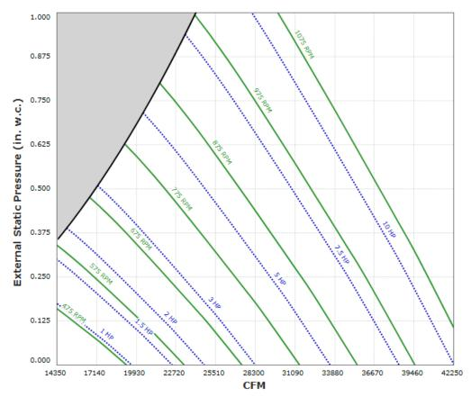
Max Sizeable RPM = 1075 RPM. Curve shown extended beyond this point for reference only.
